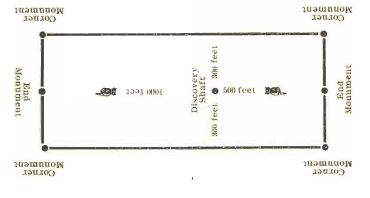
The above diagram is to give the locator a general idea of the plan of location under the new law. Your discovery shall may be in the center of claim, or any distance from either end you desire. In the diagram we have placed it 500 feet from one end and 1000 feet from the other. In description be careful to state locality of claim with reference to some natural object, or permanent monument, so as to identify the claim.
