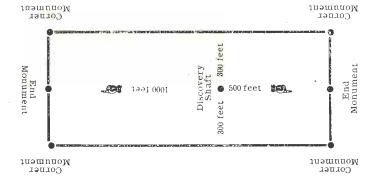
The above diagram is to give the locator a general idea of the plan of location under the new law. Your discovery shaft may be in the center of claim, or any distance from either end you desire. In the diagram we have placed it 500 feet from one end and 1000 feet from the other, in description be careful to state locality of claim with reference to some natural object, or retmanent monument, so as to identify the claim.
