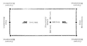
The above diagram is to give the locator a general idea of the plan of location under the new law. Your discovery shall may be in the center of claim, or any distance from either end you desire. In the diagram we have placed it 500 feet from one end and 1000 feet from the other, in description be careful to state locality of claim with reference to some natural object, or retmanent monument, so as to identify the claim.
