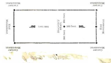
The above diagram is to give the locator a general idea of the plan of location under the new law. Your discovery shall may be in the center of claim, or any distance from either end you destre in the diagram we have placed it 500 feet from one end and 1000 feet from the claim.
