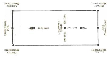
The above diagram is to give the locator a general idea of the plan of location under the new law. Your discovery shaft may be in the center of claim, or any distance from citiber end you desire. In the diagram we have placed it 500 feet from one end and 1000 feet from the other. In description be careful to state locality of claim with reference to some natural object, or permanent monument, so as to identify the claim.
