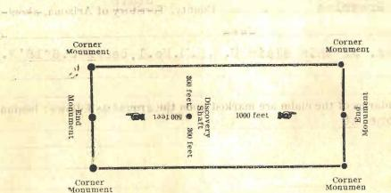
The above diagram is to give the locator a general idea of the plan or location under the new law. Your discovery shaft may be in the center of claim, or any distance from either end you desire. In the diagram we have placed it 500 feet from one end and 1000 feet from the other. In description be careful to state locality of claim with reference to some natural object, or permanent monument, so as to identify the claim.
