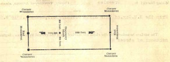
The above diagram is to give the locator a general idea of the plan of location under the new law. Your discovery shaft may be in the center of claim, or any distance from either end you desire. In the diagram we have placed it 500 feet from one end and 1000 feet from the other. In description be careful to state locality of claim with reference to some natural object, or permanent monument, so as to identify the claim.
