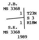
Deposit a magnet in a  $1 \times 1 \times 2$  5/8 ins. white plastic case beneath the stainless steel post.
