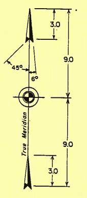
Length of Shaft - 18.0 Length of Crossbar - 3.0 ± Radius of Concentric Circles 0.5, 0.6, and 1.0
