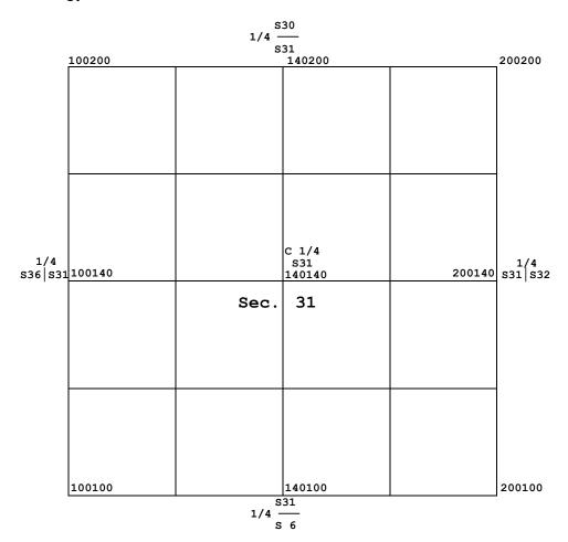
The user will notice that the four 1/4 section corners of section 31 are located at midpoint between respective section corners, and that the 1/4 section corners that fall on the east-west lines are identified with the **prefix** 140yyy, while the north-south lines have 1/4 section corners are identified by a **suffix** of xxx140.
