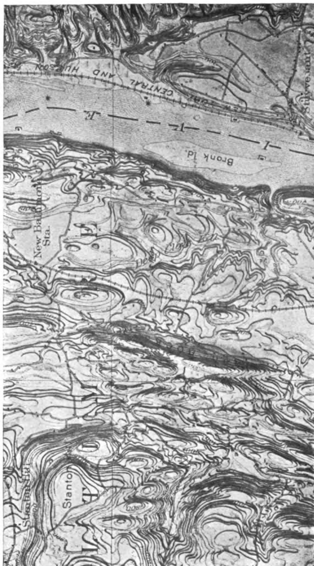
FIG. 151.—RELIEF MAP FROM CONTOUR MODEL. Scale 1 mile to 1 inch; contour interval 20 ft. Modeled by Wm. Stranahan.
