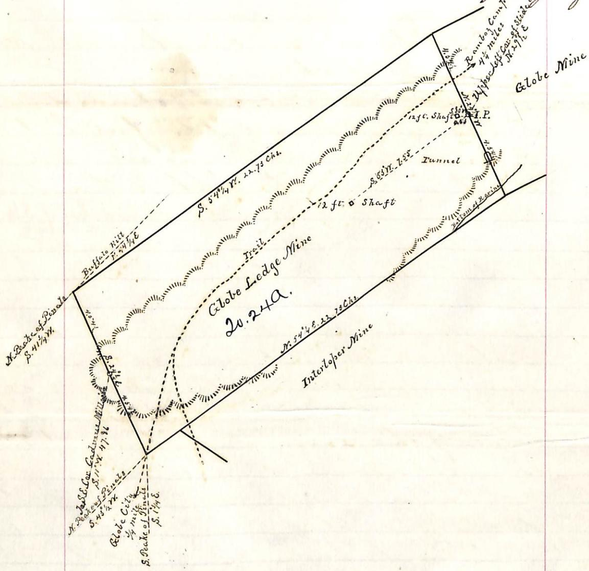
Commencing at a monument about three feet high built of copper ore and situated on the top of the Globe Hill on a large mass of Iron & Copper Croppings being the Initial Point of the Globe Ledge and Globe Mining Claims, said monument being situated about one mile North of Globe City Final Co. A. T.
