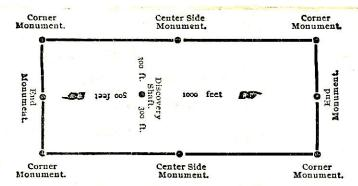
The above diagram is to give the locator a general idea of plan of location under the new law. Your discovery shaft can be in the center of taim or any distance from from either end you desire. In the diagram we have placed it 500 feet from one end and 1000 feet from the other. In lescription be careful to state locality of claim with reference to some natural object, or permanent monument, as will identify the claim.
