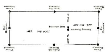
This diagram is to give locator a general idea of plan of location under the new law. The Discovery Shaft can be in the center of claim or any distance from either end desired. In the diagram it is placed 500 feet from one end and 1000 feet from the other. Commence des cription of claim at a center end monument, giving its distance and
