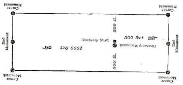
This diagram is to give location under the new law. The Discovery Shaft can be in the center of claim or sured. In the diagram it is placed 500 feet from one end and 1000 feet from the other. Commence description of claim at a center end monument, giving its distance and direction from center of Discovery Shaft; thence bound the claim in either direction. In description be careful to state locality of claim with reference to some natural object, or permanent monument, as will identify the claim.
