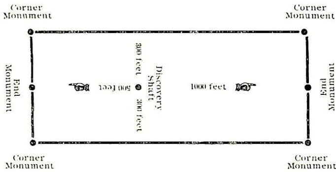
The above diagram is to give the locator a general idea of the plan of location under the new law. Your discovery shaft may be in the center of claim, or any distance from either end you desire. In the diagram we have placed it 500 feet from one end and 1000 feet from the other. In description be careful to state locality of claim with reference to some natural object, or permanent monument, so as to identify the claim.
