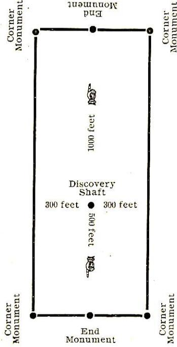
The above diagram is to give the locator a general idea of the plan of location under the new law. Your discovery shaft may be in the center of claim, or any distance from either end you desire. In the diagram we have placed it 500 feet from one end and 1000 feet from the other. In description be careful to state locality of claim with reference to some natural object, or permanent monument, so as to identify the claim.
