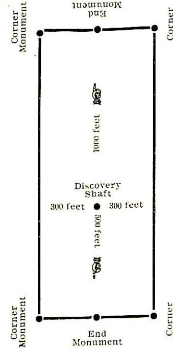
The above diagram is to give the locator a general idea of the plan of location under the new law. Your discovery shaft may be in the center of claim, or any distance from either end you desire. In the diagram we have placed it 500 feet from one end and 100 feet from the other. In description be careful to state locality of claim with reference to some natural object, or permanent monument, so as to identify the claim.
