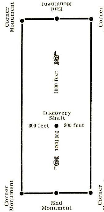
The above diagram is to give the locator a general idea of the plan of location under the new law. Your discovery shaft may be in the center of claim, or any distance from either end you desire. In the diagram we have placed it 500 feet from one end and 1000 feet from the other. In description be careful to state locality of claim with reference to some natural object, or permanent monument, so as to identify the claim.
