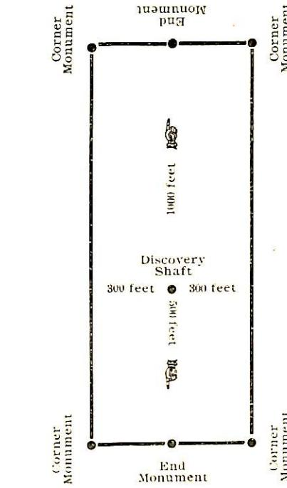
The above diagram is to give the locator a general idea of the plan of location under the new law. Your discovery shaft may be in the center of claim, or any distance from either end you desire. In the diagram we have placed it 500 feet from one end and 1000 feet from the other. In description be careful to state locality of claim with reference to some natural object, or permanent monument, so as to identify the claim.
