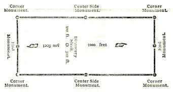
The above diagram is to give the locator a general idea of plan of location under the new law. Your discovery shaft can be in the center of staim or any distance from from either end you desire. In the diagram we have placed it 500 feet from one end and 1000 feet from the other. In description be careful to state locality of claim with reference to some natural object, or permanent monument, as will identify the claim.
