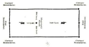
The above diagram is to give the locator a general idea of the pian of location under the new law. Your discovery shaft may be in the center of claim, or any distance from either end you desire. In the diagram we have placed it 500 feet from one end and 1000 feet from the other. In description be careful to state locality of claim with reference to some natural object, or permanent monument, so as to identify the claim.
