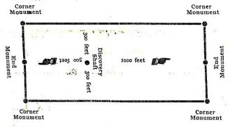
The above diagram is to give the focator a general idea of the plan of location under the new law. Your discovery shaft may be in the center of claim, or any distance from either end you desire. In the diagram we have placed it 500 feet from one end and 1000 feet from the other. In description be careful to state locative of claim with reference to some natural object from the contractive of claims.
