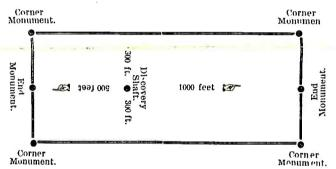
The above diagram is to give the locator a general idea of the plan of location under the new law. Your discovery shatt may be in the center of claim or any distance from either end you desire. In the diagram we have placed it 500 feet from one end and 1000 feet from the other. In description be careful to state locality of claim with reference to some natural object, or permanent monument, so as to identify the claim.
