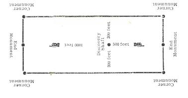
The above diagram is to give the locator a general idea of the plan of location under the new law. Your discovery shalt may be in the other, In description be careful to state locality of claim, or any distance from either end you desire. In the diagram we have placed it 500 feet from one end and 1000 feet from the other, In description be careful to state locality of claim with reference to some natural object, or permaneur, so as to identify the claim.
