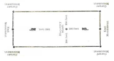
The above diagram is to give the locator a general idea of the plan of location under the new law. Your discovery shall may be in the center of claim, or any distance from either end you desire. In the diagram we have piaced it 500 feet from one end and 1000 feet from the other, in description be careful to state locality of claim with reference to some natural object, or permanent monument, so as to identify the claim.
