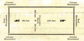
The above diagram is to give the locator a general idea of the plan of location under new law. Your discovery shaft may be in the cen'er of claim, or any distance from either end you desire. In the diagram we have placed it 500 feet from one end and 1000 feet from the other. In description, be careful to state locality of claim with reference to some natural object, or permanent monument, so as to identify the claim.
