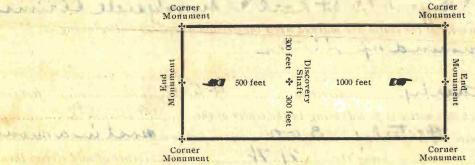
The above diagram is to give the locator a general idea of the plan of location under new law. Your discovery shaft may be in the cen'er of im, or any distance from either end you desire. In the diagram we have placed it 500 feet from one end and 1000 feet from the other. In despition, be careful to state locality of claim with reference to some natural object, or permanent monument, so as to identify the claim.
