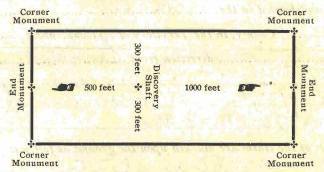
The above diagram is to give the locator a general idea of the plan of location under new law. Your discovery shaft may be n the center of claim, or any distance from either end you desire. In the diagram we have placed it 500 feet from one end and 1000 feet from the other. In description, be careful to state locality of claim with reference to some natural object, or permanent monument, so as to identify the claim.
