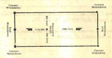
e diagram is to give the locator a general idea of the plan of location under the new law. Your discovery shaft may be in the 1, or any distance from either end you desire. In the diagram we have placed it 500 feet from one end and 1000 feet from the cription be careful to state locality of claim with reference to some natural object, or permanent monument, so as to identify the
