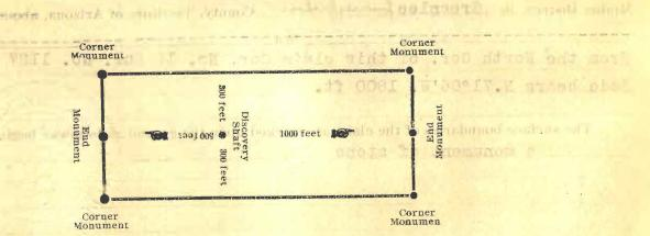
The above diagram is to give the locator a general idea of the plan of location under the new law. Your discovery shaft may be in the center of claim, or any distance from either end you desire. In the diagram we have placed it 500 feet from one end and 1900 feet from the other. In description be careful to state locality of claim with reference to some natural object, or permanent monument, so as to identify the claim.
