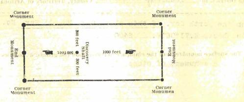
The above diagram is to give the locator a general idea of the plan of location under the new law. Your discovery shaft may be in the center of claim, or any distance from either end you desire. In the diagram we have placed it 500 feet from one end and 1000 feet from the other. In description be careful to state locality of claim with reference to some natural object, or permanent monument, so as to identify the claim.
