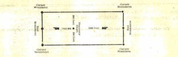
The above diagram is to give the locator a general idea of the plan of location under the new law. Your discovery shaft may be in the center of diam, or any distance from either end you desire. In the diagram we have placed it 500 feet from one end and 1000 feet from the other. In description be careful to state locality of claim with reference to some natural object, or permanent monument, so as to identify the claim.
