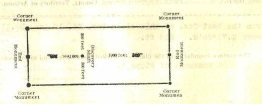
The above diagram is to give the locator a general idea of the plan of location under the new law. Your discovery shaft may be in the center of claim, or any distance from either end you desire. In the diagram we have placed it 500 feet from one end and 1000 feet from the other. In description be careful to state locality of claim with reference to some natural object, or permanent monument, so as to identify the claim.
