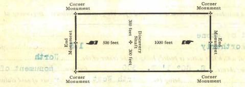
The above diagram is to give the locator a general idea of the plan of location under new law. Your discovery shaft may be in the cen'er of claim, or any distance from either end you desire. In the diagram we have placed it 500 feet from one end and 1000 feet from the other. In description, be careful to state locality of claim with reference to some natural object, or permanent monument, so as to identify the claim.
