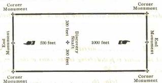
The above diagram is to give the locator a general idea of the plan of location under new law. Your discovery shaft may be in the cen'er of claim, or any distance from either end you desire. In the diagram we have placed it 500 feet from one end and 1000 feet from the other. In description, be careful to state locality of claim with reference to some natural object, or permanent monument, so as to identify the claim.
