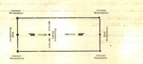
The above diagram is to give the locator a general idea of the plan of location under the new law. Your discovery shaft may be in the center of claim, or any distance from either end you desire. In the diagram we have placed it 500 feet from one end and 1000 feet from the other. In description be careful to state locality of claim with reference to some natural object, or permanent monument, so as to identify the claim.
