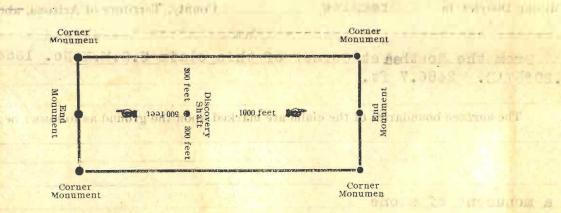
The above diagram is to give the locator a general idea of the plan of location under the new law. Your discovery shaft may be in the center of claim, or any distance from either end you desire. In the diagram we have placed it 500 feet from one end and 1000 feet from the other. In description be careful to state locality of claim with reference to some natural object, or permanent monument, so as to identify the claim.
