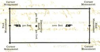
The above diagram is to give the locator a general idea of the plan of location under the new law. Your discovery shaft may be in the center of claim, or any distance from either end you desire. In the diagram we have placed it soo feet from one end and 1000 feet from the other. In description
