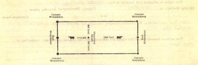
The above diagram is to give the locator a general idea of the plan of location under the new law. Your discovery shaft may be in the center of claim, or any distance from either end you desire. In the diagram we have placed it 500 feet from one end and 1000 feet from the other. In description be careful to state locality of claim with reference to some natural object, or permanent monument, so as to identify the claim.
