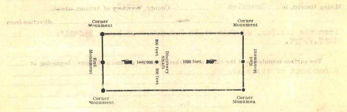
The above diagram is to give the locator a general idea of the plan of location under the new law. Your discovery shaft may be in the center of claim, or any distance from either end you desire. In the diagram we have placed it 500 feet from one end and 1000 feet from the other. In description be careful to state locality of claim with reference to some natural object, or permaneat monument, so as to identify the claim.
