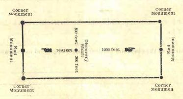
The above diagram is to give the locator a general idea of the plan of location under the new law. Your discovery shaft may be in the center of claim, or any distance from either end you desire. In the diagram we have placed it 500 feet from one end and 1000 feet from the other. In description be careful to state locality of claim with reference to some natural object, or permanent monument, so as to identify the claim.
