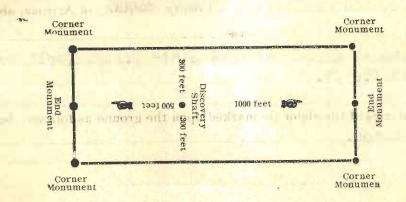
The above diagram is to give the locator a general idea of the plan of location under the new law. Your discovery shaft may be in the center of claim, or any distance from either end you desire. In the diagram we have placed it 500 feet from one end and 1000 feet from the other. In description be careful to state locality of claim with reference to some natural object, or permanent monument, so as to identify the claim.
