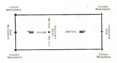
The above diagram is to give the locator a general idea of the plan of location under the new law. Your discovery shaft may be in the center of the claim, or any distance from either end you may desire. In the diagram we have placed it 500 feet from one end 1000 feet from the other. In description be careful to state locality of claim with reference to some natural object, or permanent monument, so as to identify the claim.
