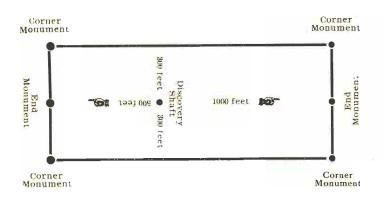
The above diagram is to give the locator a general idea of the plan of location under the new law. Your discovery shaft may be in the center of the claim, or any distance from either end you may desire. In the diagram we have placed it 500 feet from one end 1000 feet from the other. In description be careful to state locality of claim with reference to some natural object, or permanent monument, so as to identify the claim.
