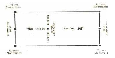
The above diagram is to give the locator a general idea of the plan of location under the new law. Your discovery shaft may be in the center of the claim, or any distance from either end you may desire. In the diagram we have placed it 500 feet from one end 1000 feet from the other. In description be careful to state locality of claim with reference to some natural object, or permanent monument, so as to identify the claim.
