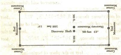
This Diagram is to give locator a general idea of plan of location under the new law. The Discovery Shaft can be in the center of the claim or any disstance from either end desired. In the diagram it is placed 500 feet from one end and 1000 ft. from the other.
