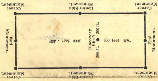
The above diagram is to give the locator a general idea of plan of location under the new law. Your discovery shaft can be in the center of claim or any distance from either end and you desire. In the diagram we have placed it 500 feet from one end and 1000 feet from the other. In description be careful to state locality of claim with reference to some natural object, or permanent monument, as will identify the claim.
