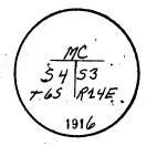
dig a pit, 36x36x12 ins., 8 ft. S. of post, and raise a mound of earth, 4 ft. base, 2 ft. high, S. of cor.
