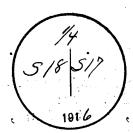
dig pits, 18x18x12 ins., N. and S. of post, 3 ft. dist.; and raise a mound of earth,  $3\frac{1}{2}$  ft. base,  $1\frac{1}{2}$  ft. high, W. of cor. Thence
