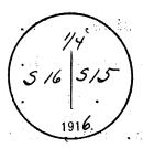
dig pits, 18x18x12 ins., N. and S. of post, 3 ft. dist.; and raise a mound of earth,  $3\frac{1}{2}$  ft. base,  $1\frac{1}{2}$  ft. high, W. of cor. Thence
