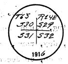
dig pits, 18x18x12 ins., in each sec.  $5\frac{1}{2}$  ft. dist.; and raise a mound of earth, 4 ft. base, 2 ft. high. W. of cor. Land, level, broken and rolling.
