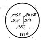
dig a pit, 36x36x12 ins., 8 ft. N. of post, and raise a mound of earth, 4 ft. base, 2 ft. high, N. of cor.
