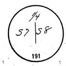
dig pits, 18x18x12 ins., N. and S. of post, 3 ft. dist.; and raise a mound of earth,  $3\frac{1}{2}$  ft. base,  $1\frac{1}{2}$  ft. high, W. of cor.
