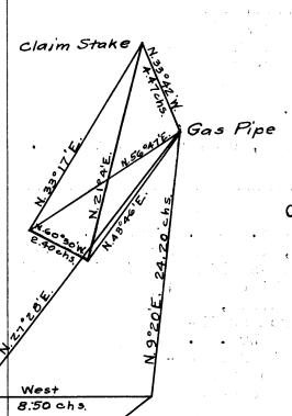
From this point a gas pipe on high spur on N. side of Diamond Creek, at the junction of Diamond Creek with the Colorado River, bears N. 9° 20' E. To determine the di To determine the dist. to this pipe, measure a base west 8.50 chs. dist. to a point from which gas pipe bears N. 27° 28' E. Tria Triangulated dist. is therefore 24.20 chs. This iron pipe has a mound of stone alongside and is about 150 ft. above the river.
