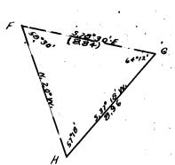
From Flag "F", triangulate as follows: Set Flag "G" on a bearing S.78°30 E. From Flag "G", measure a base \$.37°18'W., 8.96 chs. to Flag "H" from which Flag "F" bears N.20°W. The three angles of the triangle are therefore 58°30', 64°12' and 57°18', the sum of which is 180°. The distance FG is given by the sine proportion:
