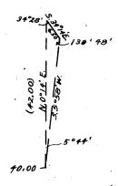
6.50 chs.--impossible to secure longer base--from the E. end of which, flag at the 1 sec. cor. of secs. 16 and 17 brs. S.5° 58'W. The three angles of the triangle are therefore 34°28', 139°48' and 5°44', the sum of which is 180°. The distance triangulated is given by the sine proportion:
