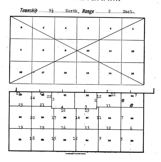
The subdivisional survey of township  $9\frac{1}{2}$  north, range 2 east, was executed with a light mountain transit made by Buff and Buff, Serial No.17992, constructed in accordance with the standard specifications of the General Land Office. For description of instrument and equipment see the field notes of the subdivisions of T.9 N., R.3 W.. surveyed under this group.
