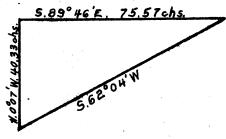
Distance by traangulation from true point for cor. of secs. 2,3,10 and 11 is 75.57 chs.
