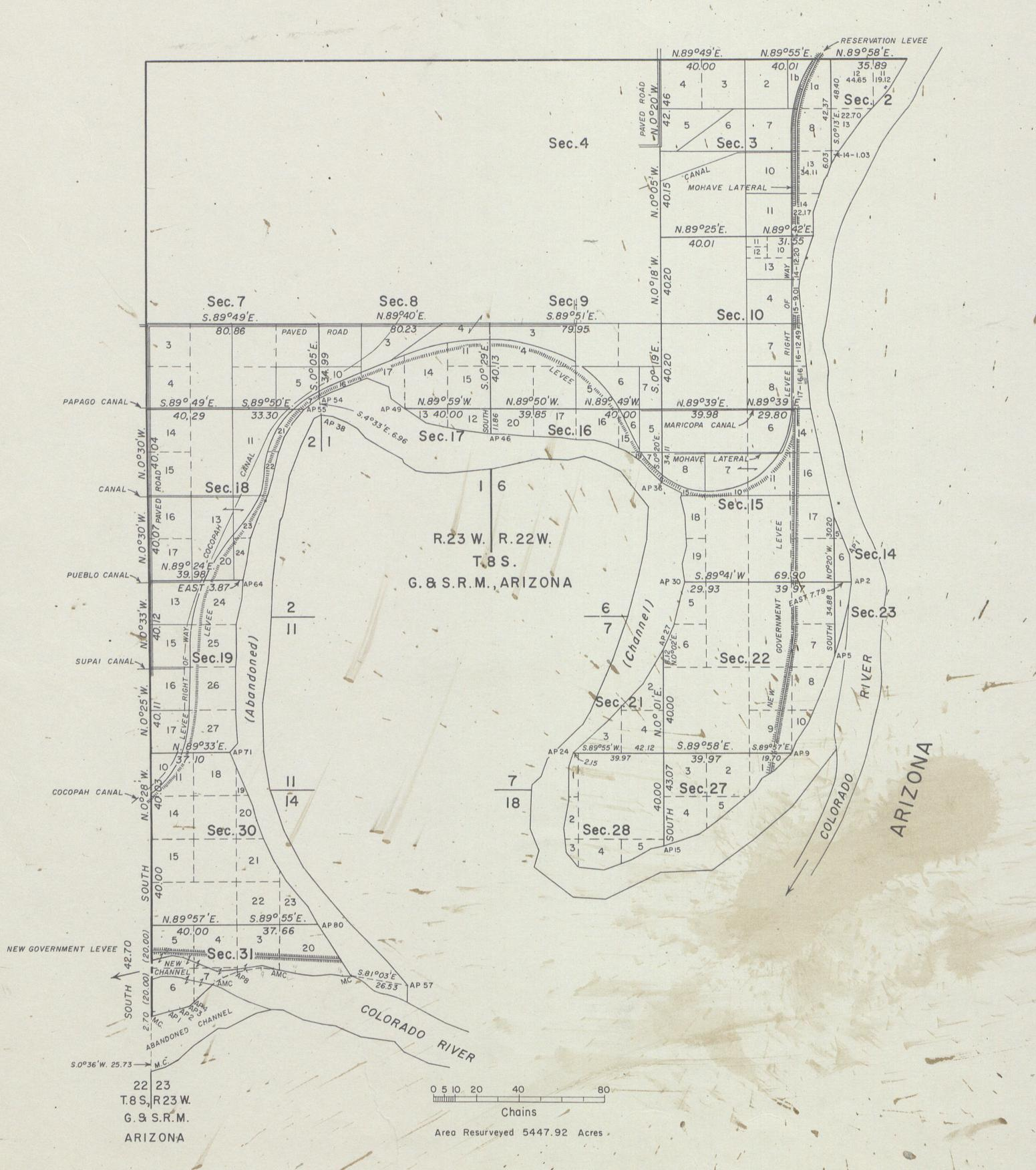
This plat represents a retracement and reestablishment of portions of the north, and west boundaries and subdivisional lines designed to restore corners thereof in their original positions according to the best available evidence.
